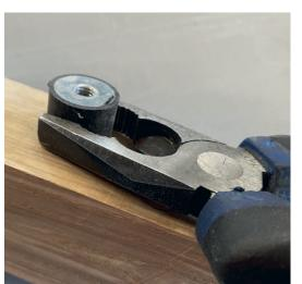
2) unscrew the defective rubber pad by hand or with pliers. As the pad's thread is coated with cement-glue, a certain amount of force is required.
